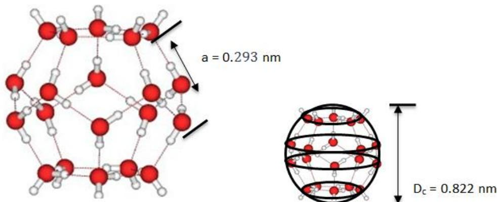
**Fig. 3.** Dodecahedral cluster with 20 water molecules at  $E=-0.1387$  eV( $\lambda = 8.95$   $\mu\text{m}$ )( $\tilde{\nu} = 1117$   $\text{cm}^{-1}$ )
